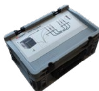
Leakage current correction HVCC VLF SIN-62
