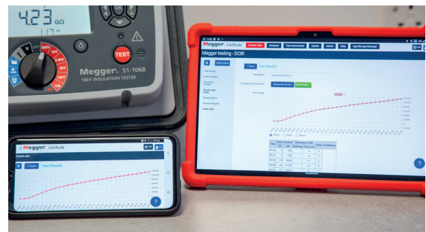
Fig 4: Ramp test current graphed live
