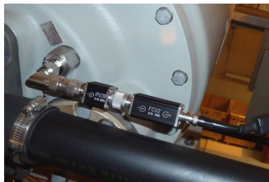
Fig. 4: External retrofit window sensors (left) and embedded sensor with IPU2B and FCU2 (right)
