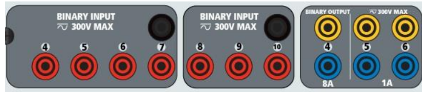
Figure 272 Binary Inputs 4 to 10 and Binary Outputs 4 to 6
