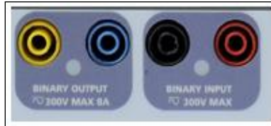
Figure 312 SMRT1 Binary Input and Output
