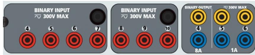
Figure 353 Binary Inputs 4 to 10 and Binary Outputs 4 to 6
