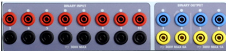
Figure 385 "P" Option Binary Inputs 3 to 10 and Binary Outputs 3 to 6
