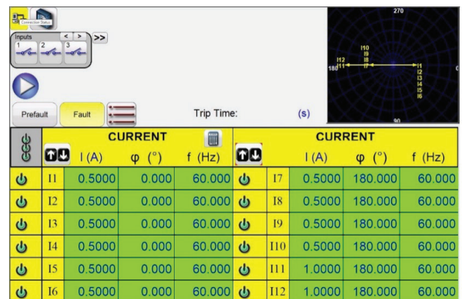
Figure 33: 12-Currents Simulating Bus Differential Scheme
