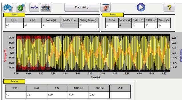
Figure 39: Power Swing Input Setting Screen and Waveforms
